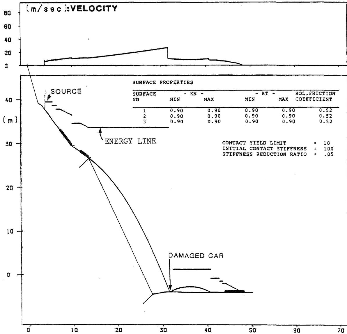
Figure 11 Dynamic analysis of the trajectory of the 1982 rockfall accident north of Porteau.
