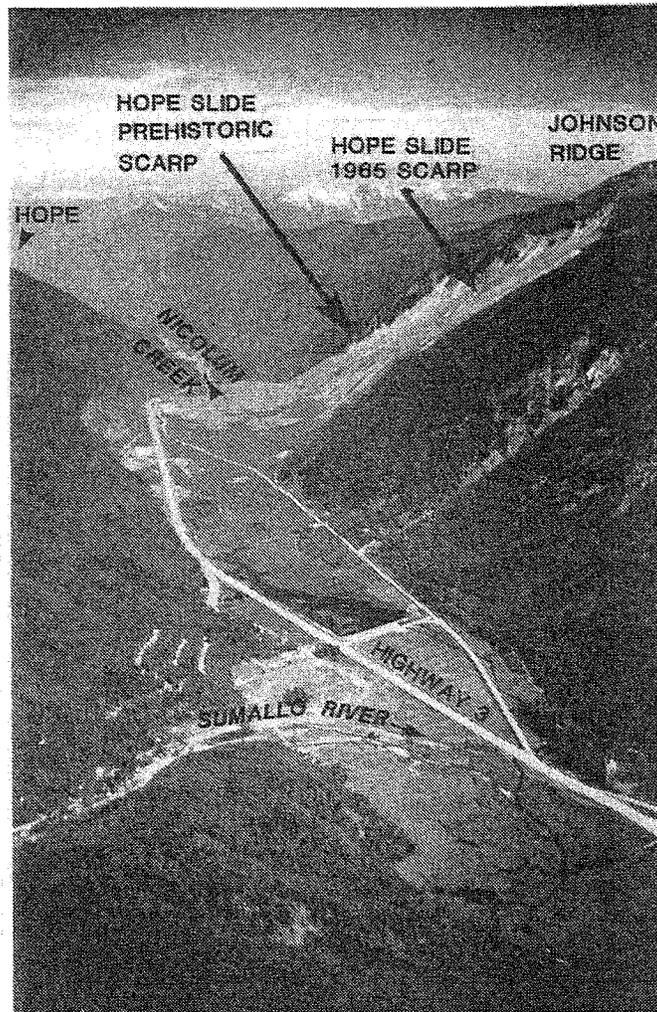
Figure 17: Hope Slide is the only historical rock avalanche in the vicinity of the lower Fraser River valley transportation corridor. On January 9, 1965, approximately 50 million cubic metres of rock and snow inundated the Nicolum-Sumallo valley, burying Provincial Highway 3. The slide occurred in the headscarp of a prehistoric slide of similar magnitude (from Savigny, 1992).
