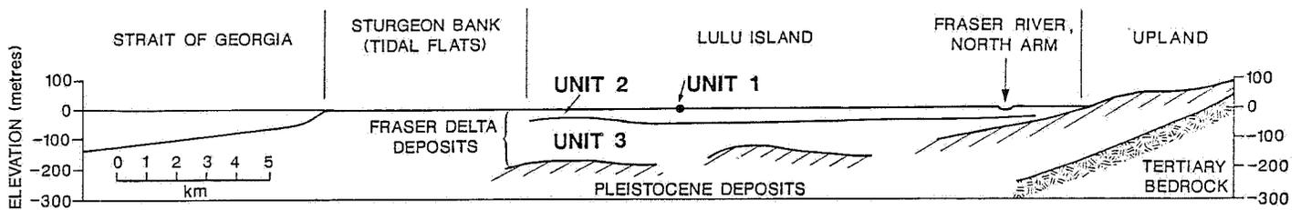
Figure 3. Fraser Delta Stratigraphic Section.
