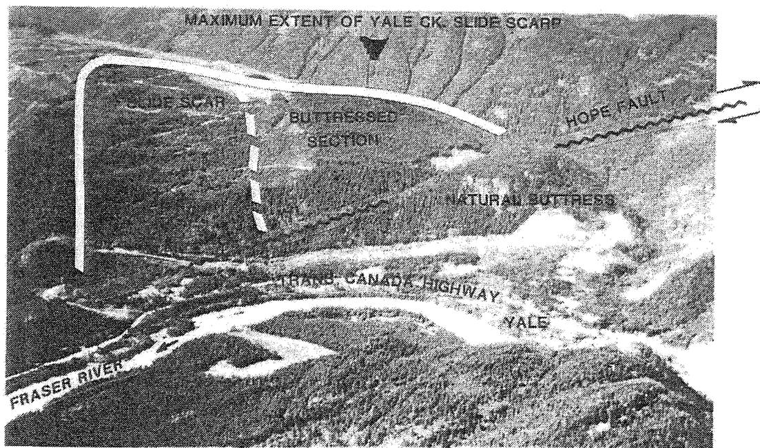
Figure 24: Low level oblique aerial photograph of the suspected Yale Slide (from Savigny, 1992).
