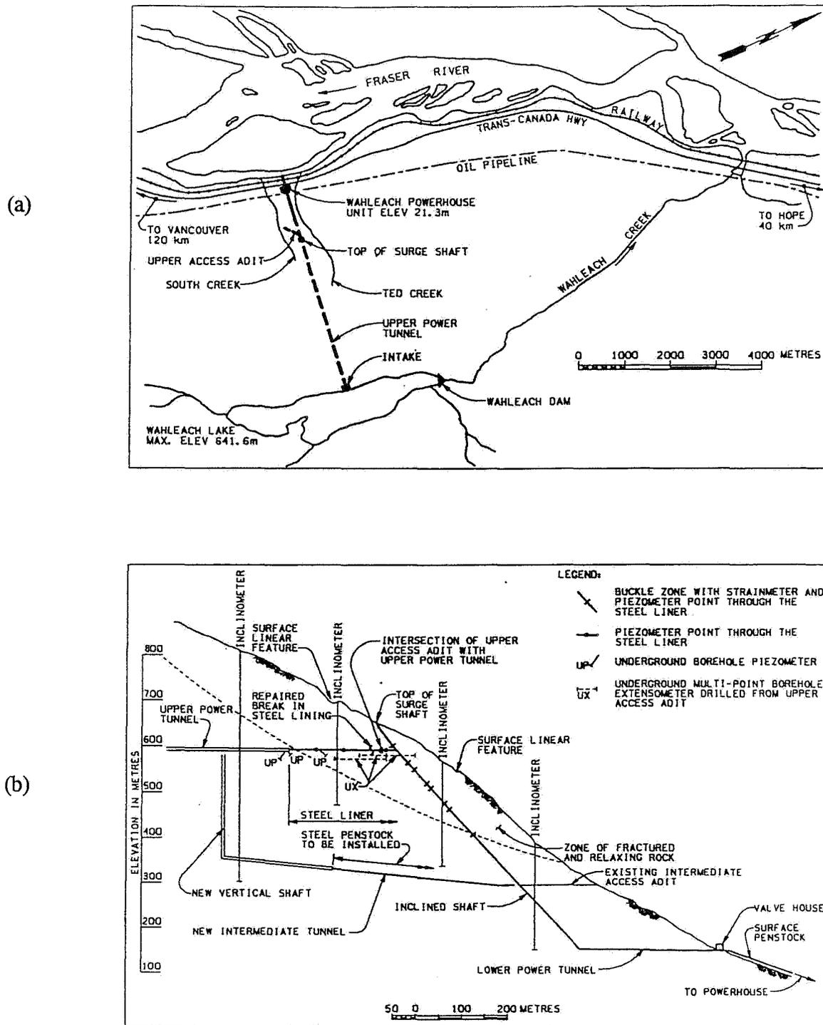
Figure 13: Wahleach Project: a) Layout. b) Cross-section looking west. The dashed line is the approximate location of a gradational boundary between loosened, fractured and weathered rock and more intact rock. Downslope movement - currently being monitored - is generally well above this boundary (from Moore *et al.*, 1991).
