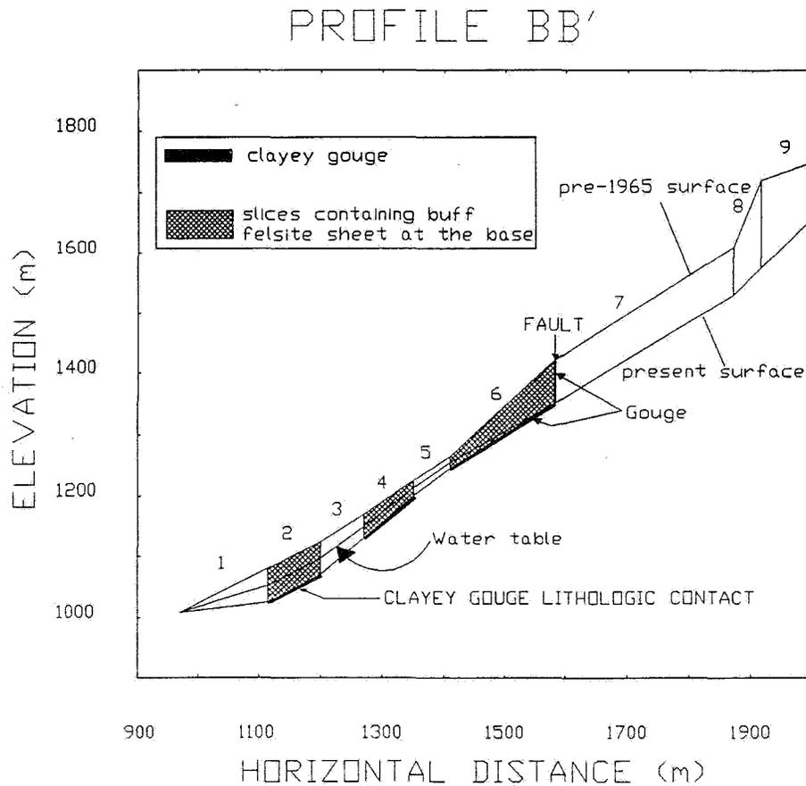
Figure 23: Cross-section BB' used in back analysis (from von Sacken, 1991).
