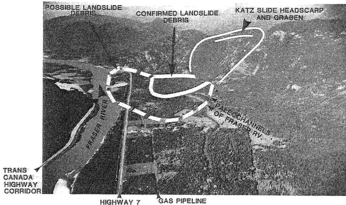
Figure 16: An oblique air photo looking downstream along the lower Fraser River valley transportation corridor in the vicinity of Katz Slide (from Savigny, 1992).
