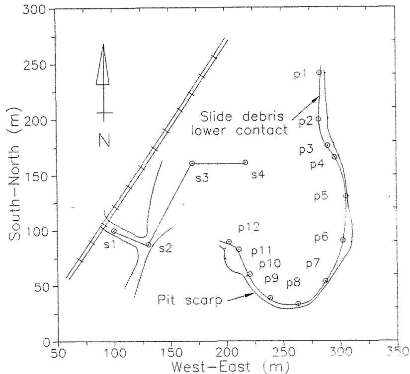
Figure 9: Map of the CN Rail gravel pit showing survey stations at the lower slide debris contact (coded 'P') in the working face exposures, and the survey line used to bring elevation control from the CN Rail tracks (coded 'S'). Corresponding vertical sections are shown in Figure 10. Note, the position of the working face is depicted as of August 1989. The location of the pit in the Cheam Slide debris is shown on Figure 7 (from Naumann, 1990).
