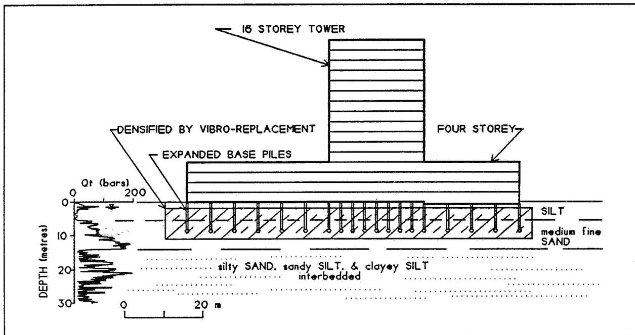
Figure 7. Typical Section (Westminster Highway and No. 3 Road)
