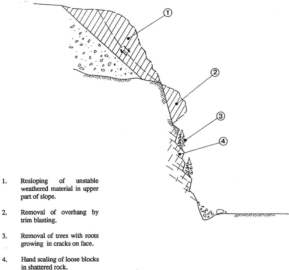
Figure 28: Rock removal methods for slope stabilization.
