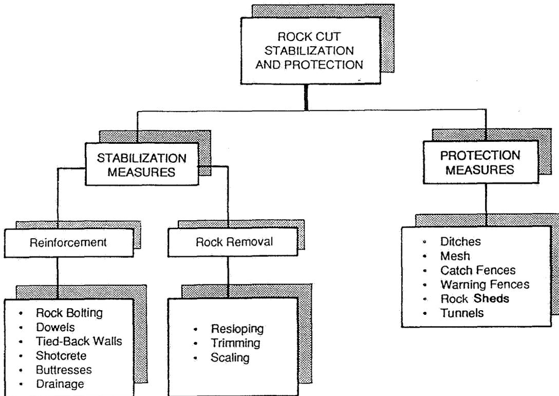
Figure 26: Classes of rock slope stabilization measures.
