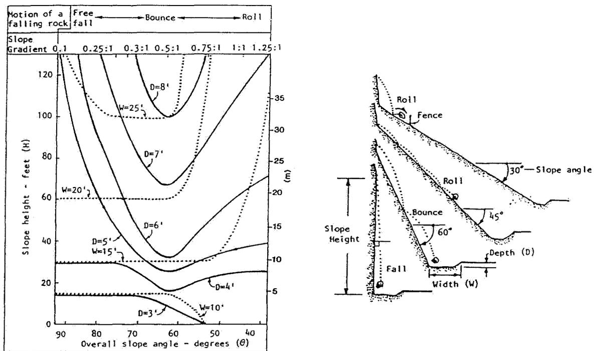
Figure 29: Design chart to determine the required width and depth of rock catch ditches in relation to the height and face angle of the slope (from Ritchie, 1963).
